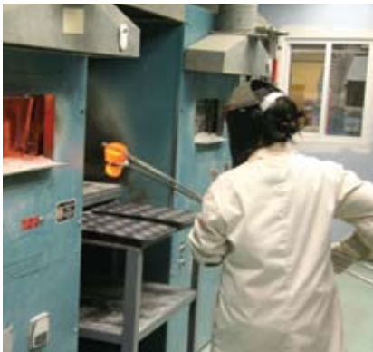
Assay Technician at Troilus preparing a sample for gold pyroanalysis (fire assay).
