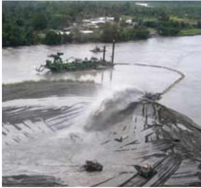
Close-up of the large dredge moving tailings from the river downstream of Ok Tedi.
